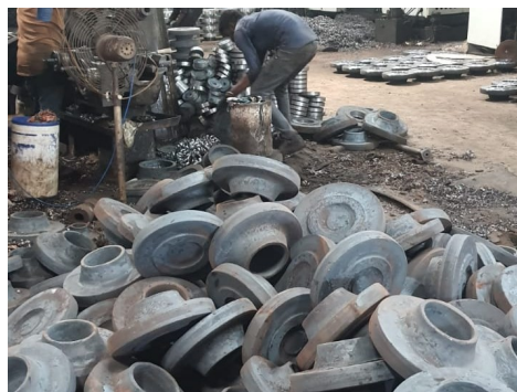
BLANKS OFF THE HAMMER
