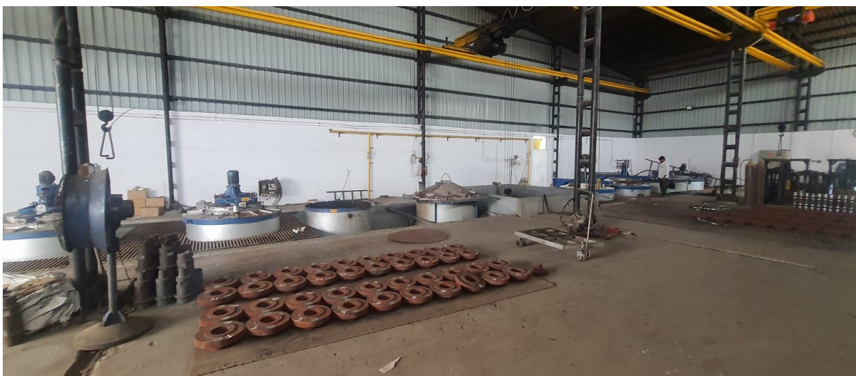
NORMALISED, AWAITING MACHINING
