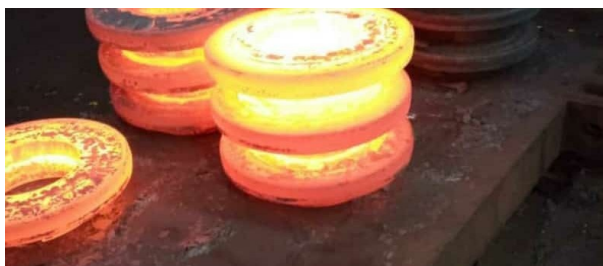
FORGED RINGS, COOLING
