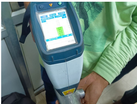
POSITIVE MATERIAL IDENTIFICATION
