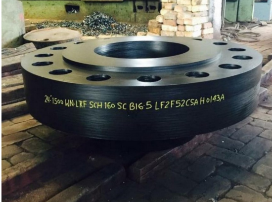
MARKED TO MSS SP-25
