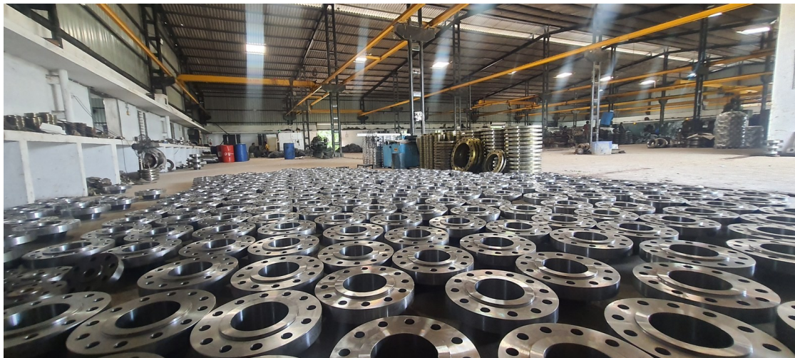
FINISHED FLANGES AWAITING MARKING
