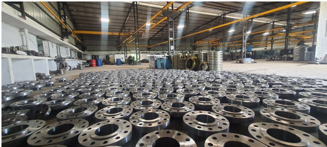
FINISHED FLANGES AWAITING MARKING
